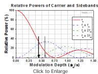
Figure 3: Curves Relating the Power in the Carrier and Several Sideband Peaks as A Function of Modulatrion Depth
