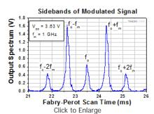
Figure 4: EO Phase Modulator Spectrum When V<sub>pp</sub> = 3.63 V
